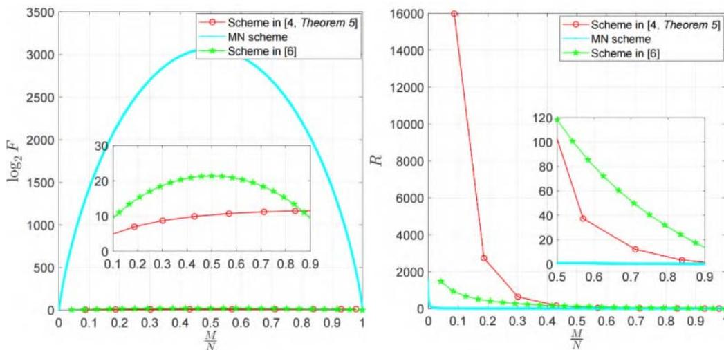
Fig. 2: Subpacketization level and transmission rate comparison between the schemes in *Theorem 5, [6]* and the MN scheme, where  $K=3072$ .
