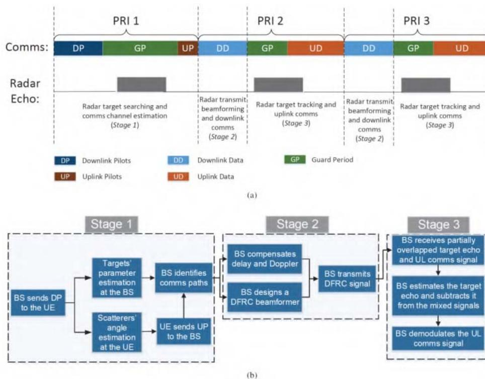
Fig. 1. The proposed DFRC signal frame structure and signal processing flow chart.
