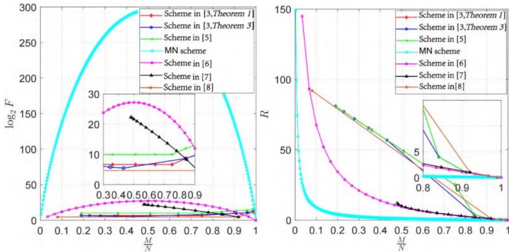
Fig. 1: Subpacketization level and transmission rate comparison between the schemes in *Theorems 1, 3, [5-8]* and the MN scheme, where  $K=300$ .
