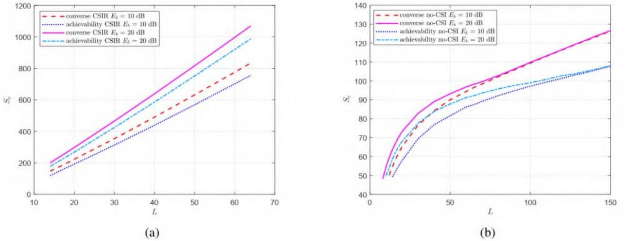
Fig. 2: The spectral efficiency versus  $L$  with  $n = 1000$ ,  $J = 100$ ,  $\frac{\kappa a}{\kappa} = 0.4$ , and  $\epsilon = 10^{-3}$ : (a) CSIR; (b) no-CSI.
